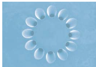
Fuel injector holes need to be smaller than ever and drilled into complex shapes.
