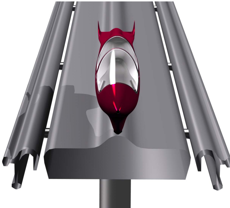
Fig. 21: Raised center of the track profile for further system optimization c_d=0,05 , 200 mph at 14 KW, two passengers and 132 mpg
