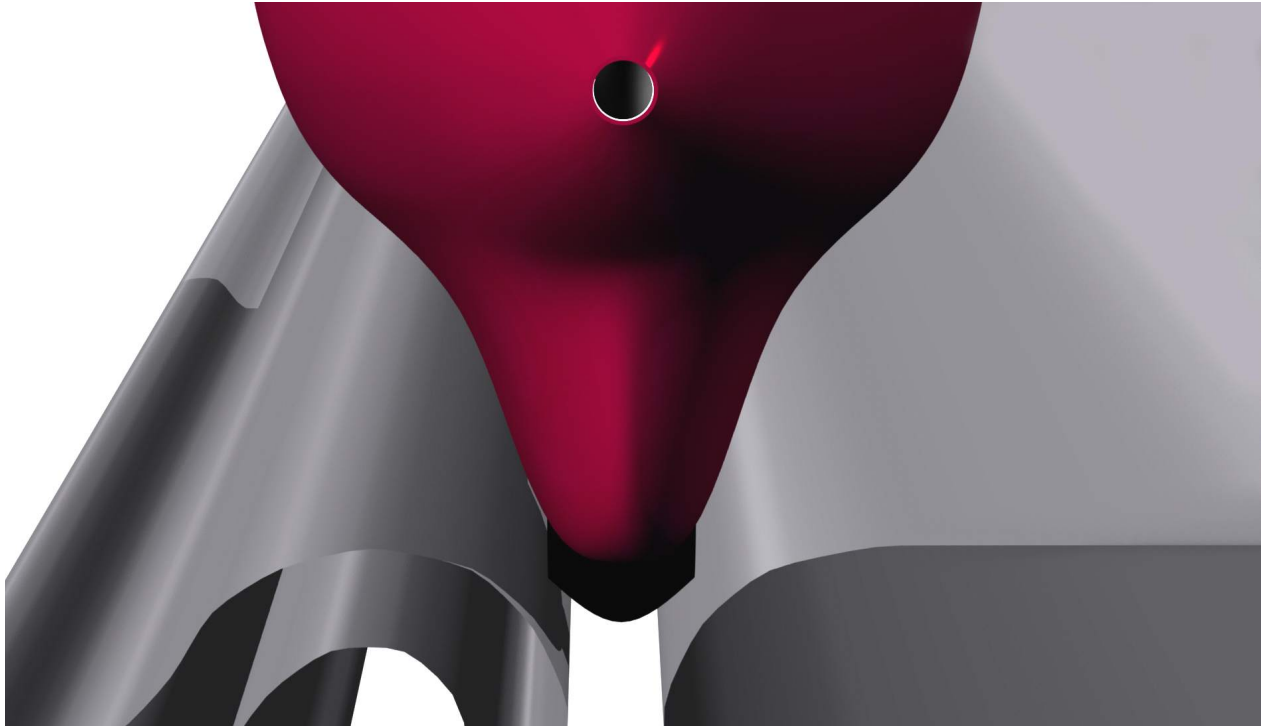
Fig. 19: Acabion with pendulum and aerodynamic-balance in the V-rail
