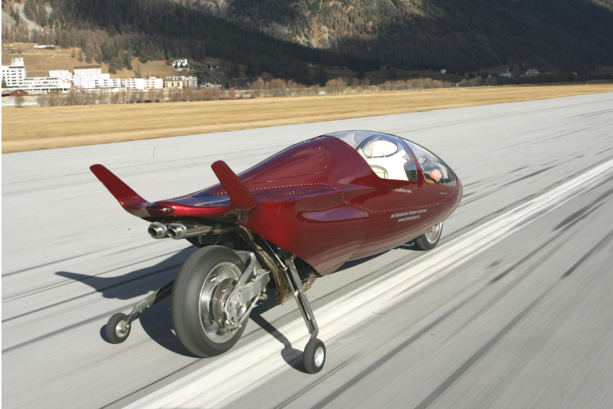
Fig. 12: Acabion GTBO test drive at Samedan / St. Moritz airport, Side-wheel tests at 50...70 mph
